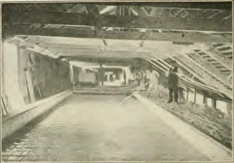
FIG. 12. CLAY KILN, SHOWING SCORING INTO RECTANGULAR BLOCKS. (Photo, English China Clays, Ltd., St. Austell).
